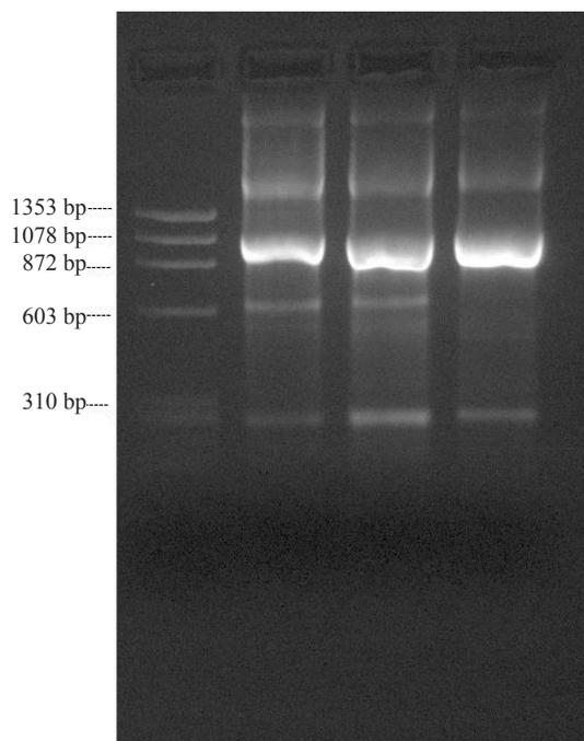
Figure 3. Amplified pab fragment from chromosomal DNA of *M. tuberculosis*. Lanes: 1= DNA marker; 2-4= amplified pab gene correspond to 970 bp.
